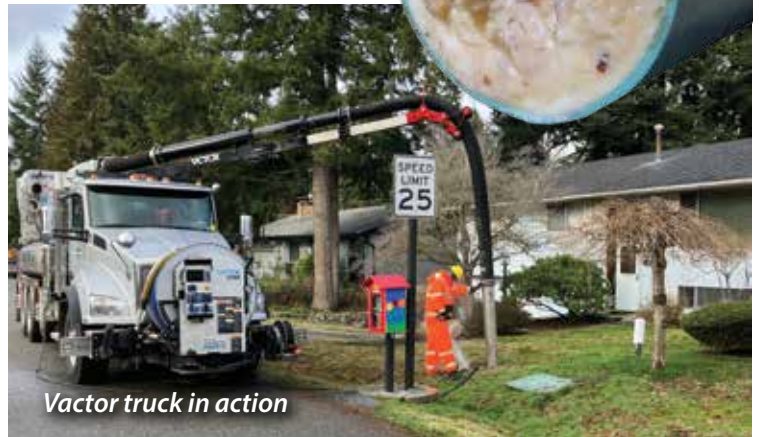
Sewer line clogged by fats, oils, and grease (often exacerbated by [non]-"flushable" wipes)
