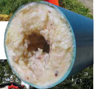
Sewer line clogged by fats, oils, and grease (often exacerbated by [non]-"flushable" wipes)
