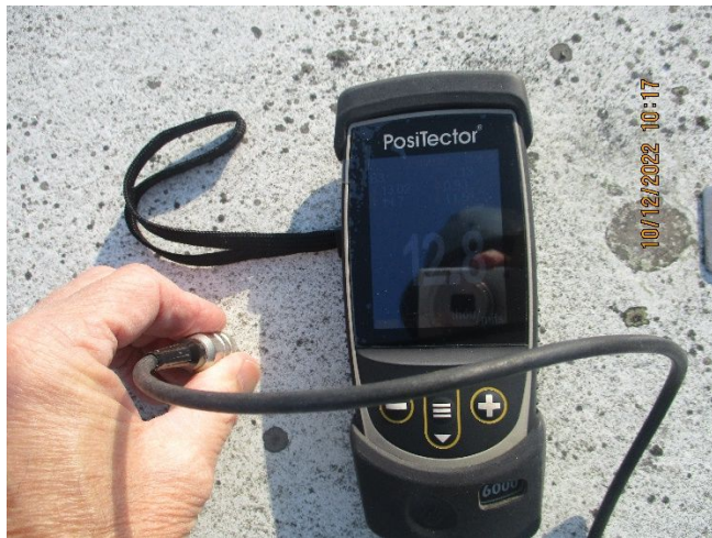
PHOTO 6 Dry Film Thickness Measurement
